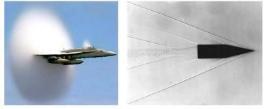
*a)* Oblique shock wave at a supersonic aircraft. An expansion upstream of the shock wave results in a decrease in temperature and condensation of water vapour.
